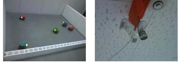
Fig. 3. Field (left) and the USB camera on the ceiling (right) of the environment of the experiments. For the field, the top leftmost corner is the origin; and x and y axes are along the thermocol blocks and the wall, respectively.
